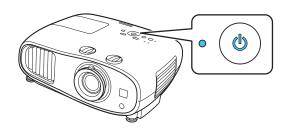
**Note:** To shut down the projector, press the  $\bigcirc$  power button on the projector twice or the  $\bigcirc$  **Standby** button on the remote control once. You don't have to wait for the projector to cool down.
