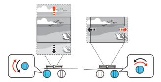
If the image is tilted, adjust the front feet as shown below.
