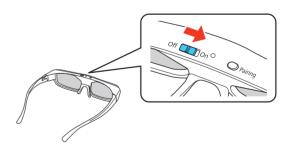
**Note:** If the glasses don't automatically display 3D content, you may need to pair them with the projector. Move the glasses within 10 feet (3 m) of the projector, then press and hold the **Pairing** button on the 3D glasses for at least 3 seconds. The status light on the glasses will alternately flash green and red, then remain green for 10 seconds if pairing is successful.
