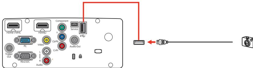
**Note:** Do not connect a USB hub or a USB cable longer than 10 feet (3 m), or the device may not operate correctly.
