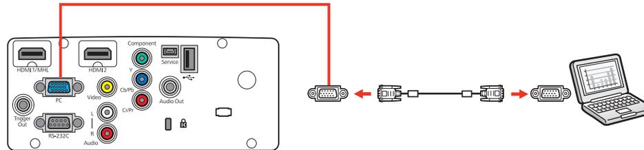
4. Tighten the screws on the VGA connector.
