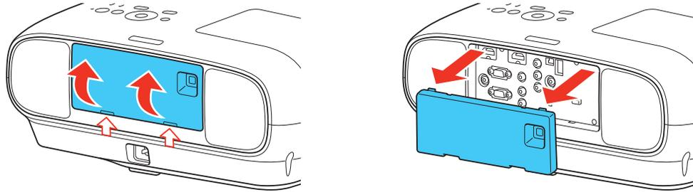
To attach the cable cover, insert the top end first, then push the cable cover in.
