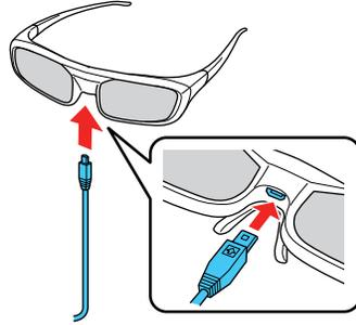
**Note:** Make sure you connect the cable in the correct orientation or you may damage the glasses or cable.
