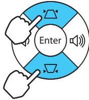
3. Press a keystone button on the projector's control panel to adjust the image shape.
