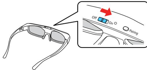
5. Move the glasses within 10 feet (3 m) of the projector, then hold down the **Pairing** button on the glasses for at least three seconds.
