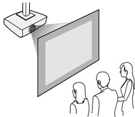
Wherever you set up the projector, make sure to position it squarely in front of the center of the screen, not at an angle, if possible. If the projector cannot be centered in front of the screen, use lens shift to reposition the image instead of using keystone correction for better image quality.
