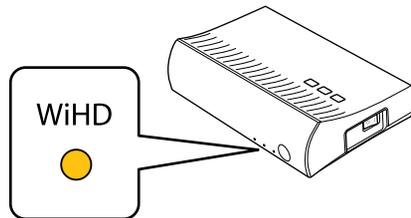
**Note:** If the WirelessHD connection fails, press the **Setup** button on the bottom of the WirelessHD transmitter and try again.
