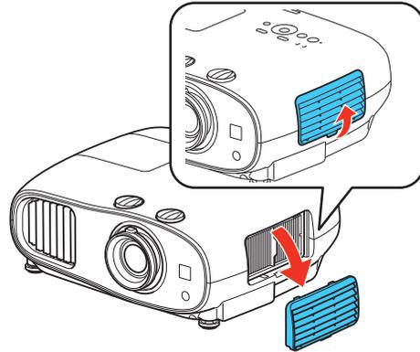
3. Pull the air filter out of the projector.
