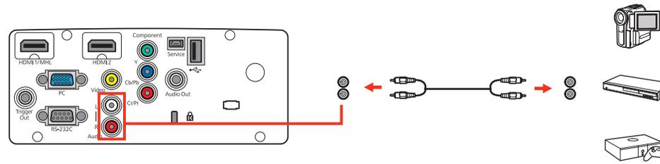
**Note:** To add additional sound, connect your video source and speakers to an audio video receiver, then connect the receiver to the projector using one of the receiver's compatible video outputs (an HDMI connection provides the best image quality, if available). You can also connect speakers to any video source that has its own speaker connections. You can also connect externally powered speakers or headphones to the **Audio Out** port using a 3.5 mm stereo mini jack cable.
