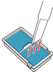
**Note:** If dust is difficult to remove or the air filter is damaged, replace the air filter.
