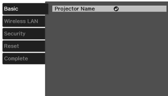
6. Select the **Projector Name** setting and enter a name up to 16 alphanumeric characters long to identify the projector over the network.
