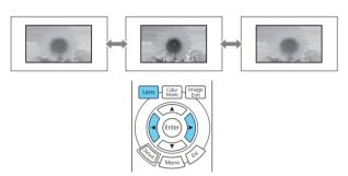
4 Press the Lens button on the remote control again and use the ◀ and ► buttons to reduce or enlarge the image.
