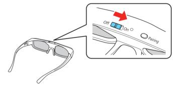
**Note:** If the glasses don't automatically display 3D content, you may need to pair them with the projector. Move the glasses within 10 feet (3 m) of the projector, then press and hold the **Pairing** button on the 3D glasses for at least 3 seconds. The status light on the glasses will alternately flash green and red, then remain green for 10 seconds if pairing is successful.
