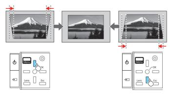
**Note:** Using the keystone adjustment can affect the size and effective resolution of your image. If possible, change the position of your projector to eliminate the keystone effect and use the lens shift option to position the image as necessary.
