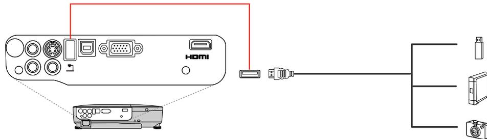
**Note:** Do not connect a USB hub or a USB cable longer than 10 feet (3 m), or the device may not operate correctly.
