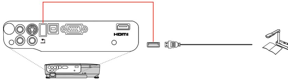
3. Connect the other end of the cable to the document camera's USB Type B port.
