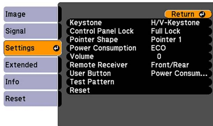
3. Select the **Control Panel Lock** setting and press **Enter**.
