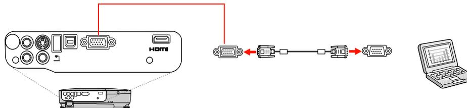
4. Tighten the screws on the VGA connectors.
