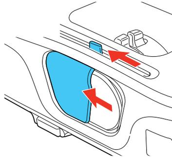
2. To cover the lens or temporarily turn off the projected picture and sound, slide the **AV Mute** slide cover closed.
