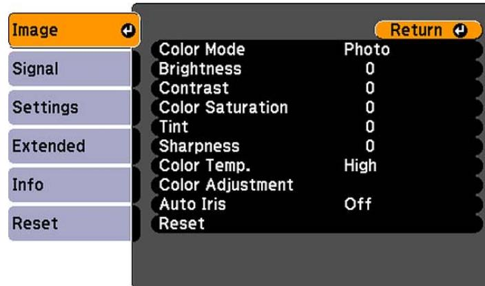
2. Press the up or down arrow buttons to move through the menus listed on the left. The settings for each menu are displayed on the right.
