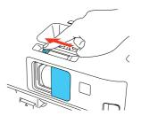
4 Press the opower button on the projector or remote control. The projector beeps, the Status light flashes blue, and then stays on.
