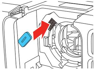
3. Slide the lock lever to the **Release** position (as shown) until you hear it click.
