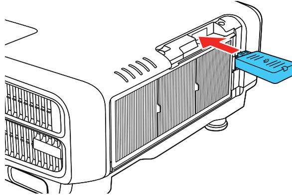
5. Replace the wireless LAN module stopper and secure it using the screw you removed.
