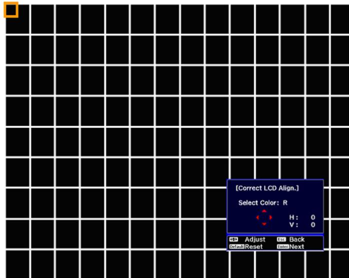
11. Use the arrow buttons on the remote control to adjust the color alignment in the corner of the screen highlighted by the orange box.
