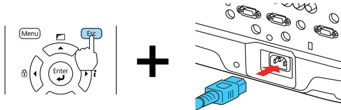
5. When the On/Standby and Status lights are blue, and the Laser and Temp lights are orange, release the **Esc** button.
