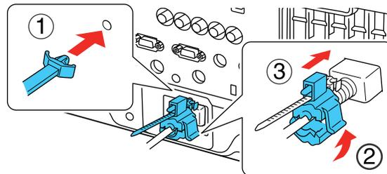
3. Place the open cable clip around the power cable, but don't lock it into place.
