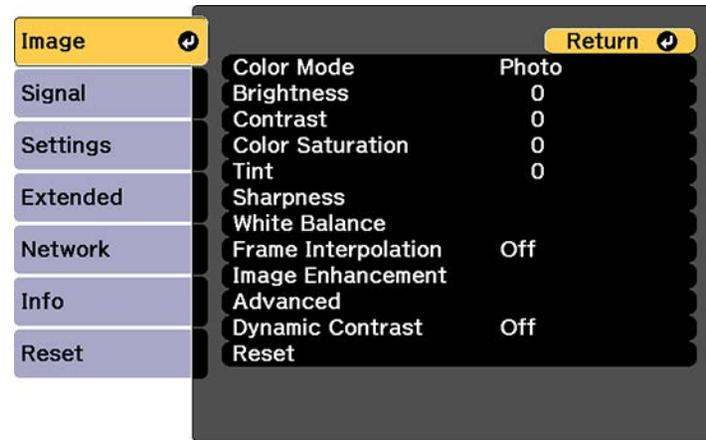
2. Press the up or down arrow button to move through the menus listed on the left. The settings for each menu are displayed on the right.
