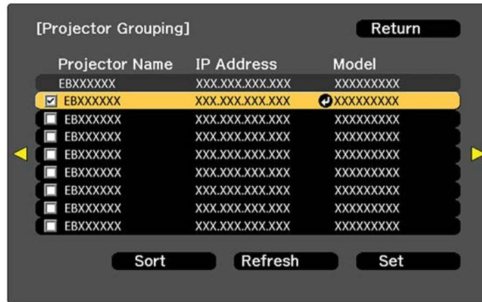
6. Press the up or down arrow buttons to highlight a projector and press **Enter** to place a checkmark next to each projector you want to use for tiling. Then select **Set** and press **Enter**.
