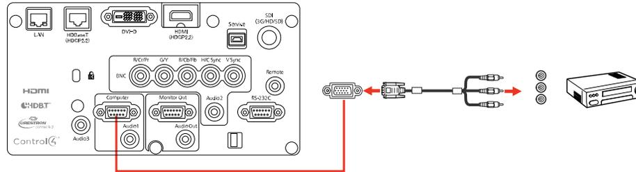
3. Tighten the screws on the VGA connector.
