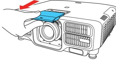
4. Hold the lens firmly as you slide the lock lever to the **Release** position (as shown) until you hear it click.
