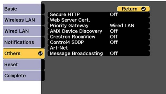
5. If you want to use the Secure HTTP protocol to encrypt communication when using Web Control, turn on the **Secure HTTP** setting and import the web server certificate using the **Web Server Cert.** setting.
