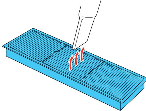
**Note:** If dust is difficult to remove or the air filter is damaged, replace the air filter.
