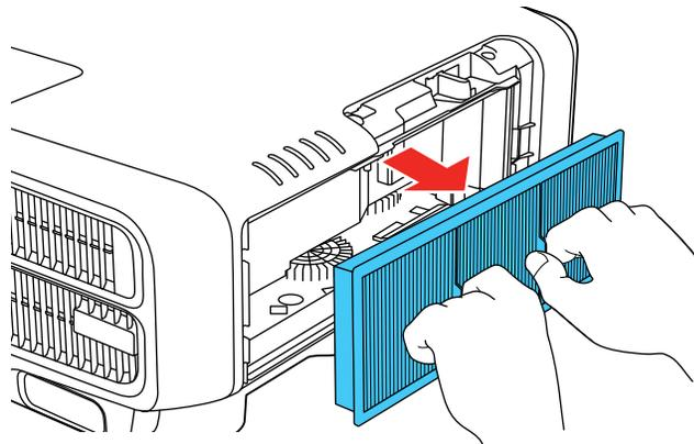
**Note:** Air filters contain polypropylene. Dispose of used air filters according to local regulations.
