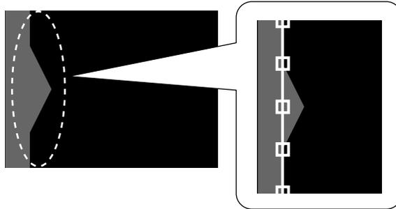
14. Use the arrow buttons to adjust the boundary line position and press the **Enter** button.
