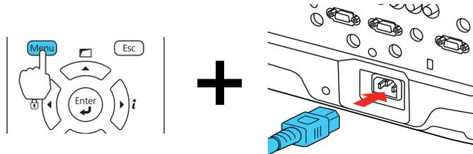
4. When the On/Standby and Status lights are blue, and the Laser and Temp lights are orange, release the **Menu** button.
