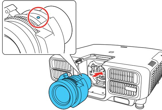
5. Hold the lens firmly and slide the lock lever to the **Lock** position (as shown) until it locks.
