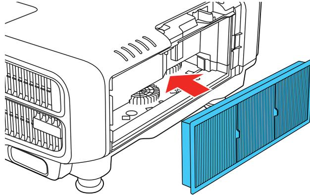
5. Attach the air filter cover as shown, and press it gently until it clicks into place.
