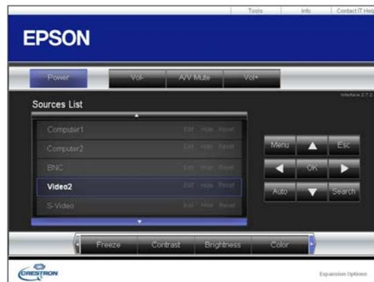
3. Select the input source that you want to control in the Sources List box. You can scroll through available sources using the up and down arrows in the box.
