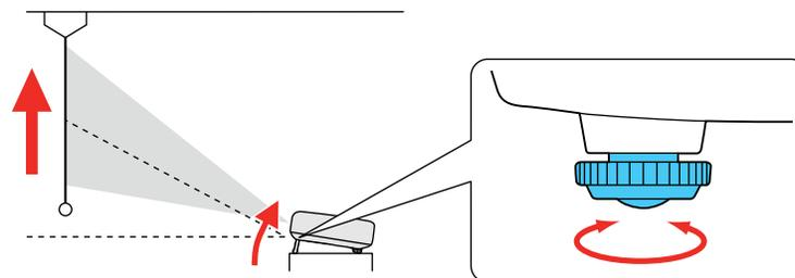
3. If the image is tilted, rotate the rear feet to adjust their height.
