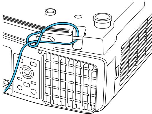
**Note:** Do not pass drop-prevention cables through the security cable attachment point when mounting the projector on a wall or ceiling.
