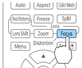
3. Press and hold the arrow buttons on the projector's control panel or remote control to adjust the focus.
