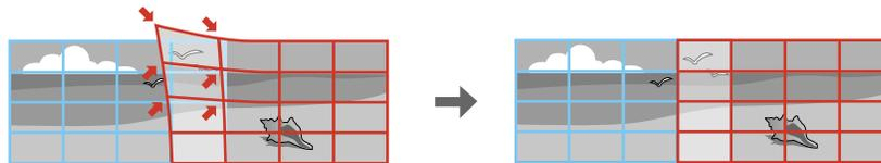
**Note:** You can move the points on the grid between 0.5 to 32 pixels for WUXGA models or 0.5 to 27 pixels for SXGA+ models in any direction. If you see a 4K Enhancement message, select **Yes** to disable the 4K Enhancement feature.
