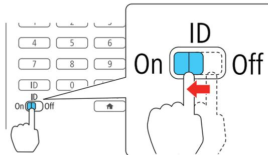
3. Hold down the **ID** button on the remote control while you press the numeric button that matches the projector's ID. Then release the buttons.
