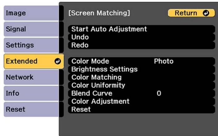
When adjustment starts, you see an adjustment pattern. Adjustment is complete when you see a displayed image.
