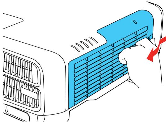
3. Pull the air filter out of the projector.
