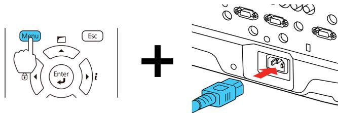
5. When the On/Standby and Status lights are blue, and the Laser and Temp lights are orange, release the **Menu** button.
