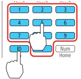
**Note:** If you don't know the projector's ID, hold down the **ID** button and press the **Home** button to temporarily display the projector's ID on the screen. If the batteries are left out of the remote control for an extended period, the remote control ID returns to its default setting.
