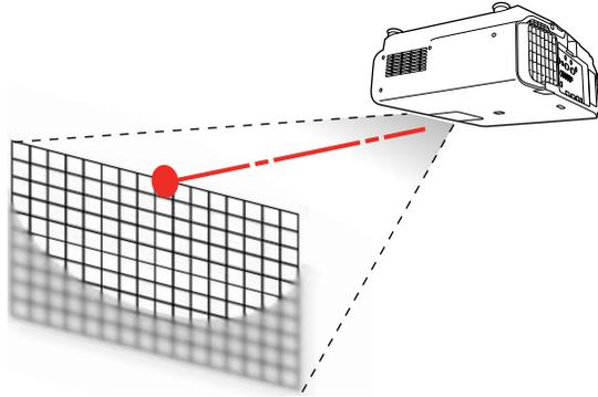
4. Press the **Focus** button on the remote control or press the **Lens** button on the control panel repeatedly until the distortion adjustment screen appears.
