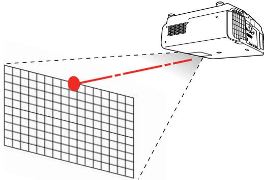
**Note:** If you installed the optional ELPLU02 short throw lens and you see a message prompting you to manually adjust the image distortion, manually rotate the distortion ring counterclockwise. Adjust the focus and then rotate the distortion ring again to correct image distortion.
