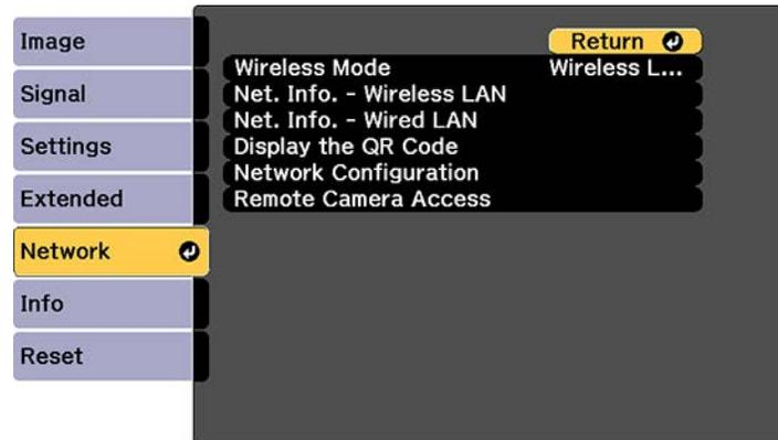
5. Make sure the **Secure HTTP** setting is enabled by selecting **Network Configuration > Others > Secure HTTP > On**, then return to the Network menu.
