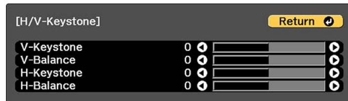
6. Use the arrow buttons on the projector or the remote control to select between vertical and horizontal keystone correction and to adjust the image shape as necessary.
