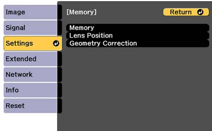
**Note:** You can also access this screen by pressing the **Memory** button on the remote control.
