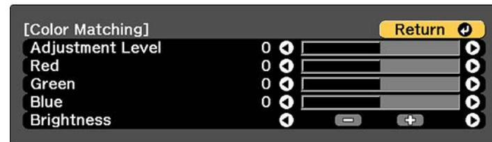
6. Press the left or right arrow buttons to select a value for the **Adjustment Level** setting.
