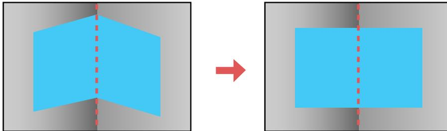
**Note:** For the best results, project from the front of the screen onto a right-angled surface and with the lens in the home position. The image may not be evenly focused throughout even after performing the steps here. If you see a 4K Enhancement message, select **Yes** to disable the 4K Enhancement feature. Corner Wall is not supported for the ELPLX02 lens.
