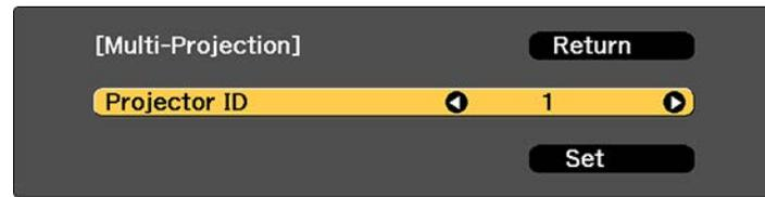
5. Press the left or right arrow buttons on the remote control to select the identification number you want to use for the projector. Then select **Set** and press **Enter**.
