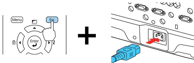
4. When the On/Standby and Status lights are blue, and the Laser and Temp lights are orange, release the **Esc** button.
