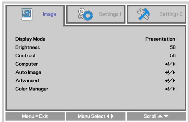
2. Press the ◀▶ buttons to move to the **Settings 1** menu. Press the ▲▼ buttons to select **Advanced 1**.
