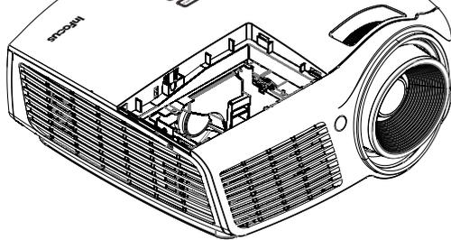
5. Pull firmly on the module handle to remove the lamp module.
