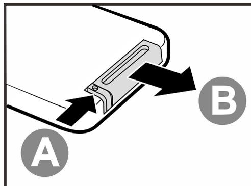
2. Insert a 3V lithium battery with the positive side facing up.
