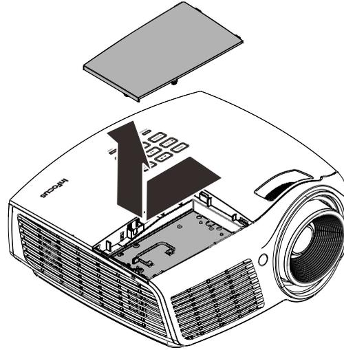
3. Remove the three screws from the lamp module.
