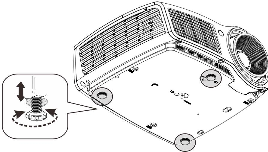
To adjust the angle of the picture, turn the tilt-adjuster right or left until the desired angle has been achieved.
