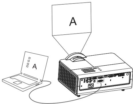
Change the Multiple Display setting to "Duplicate these displays" (Windows 7: Control Panel > Display > Screen Resolution). Varies per operating system.
