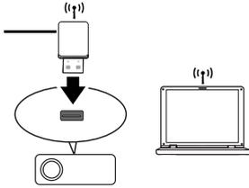
To connect to the projector wirelessly, you need to plug an optional InFocus wireless dongle (p/n SP-WIFIUSB) to the USB Type A connector on the projector, and then check the Wireless LAN Info on Network Info menu.
