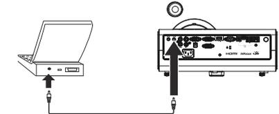
If you are using a desktop computer and want to see the image on your computer screen as well as on the projection screen, connect to the desktop's computer cable to Computer 1 and the desktop's monitor cable to the **Monitor out** connector on the projector.
