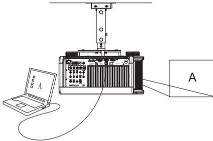
DisplayLink - Use DisplayLink software to change the display mode from Extended Desktop to Duplicated Desktop. Windows - Disable “Extend my Windows Desktop” in Control Panel > Display > Settings > Display 2 (location varies by operating system).
