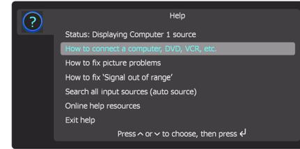
**NOTE:** The projector can be re-programmed to display a custom (non-interactive) screen when Help is pressed. To do this: Create your custom screen on a computer and display it on the projector, then use the Take Snapshot command in the Setup menu. When you see the Snapshot Successful message, hold down the Help button until the message is removed.
