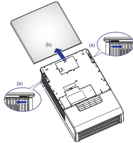
2 Loosen the four screws then lift the lens door.
