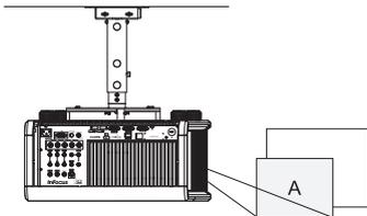
Adjust Lens Shift in the Basic Picture menu.
