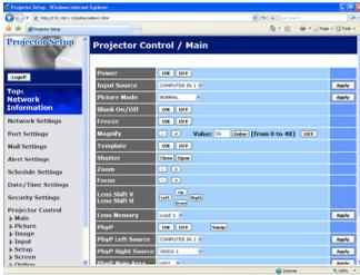
The items shown in the table below can be performed using the Projector Control menu. Select an item using the up and down arrow keys on the PC.
