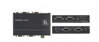
The VP-211K is a high-performance switcher for computer graphics video signals, with resolutions up to and exceeding UXGA, and unbalanced stereo audio signals. When configured as a standby switcher, it switches to the secondary input upon loss of the primary input.
