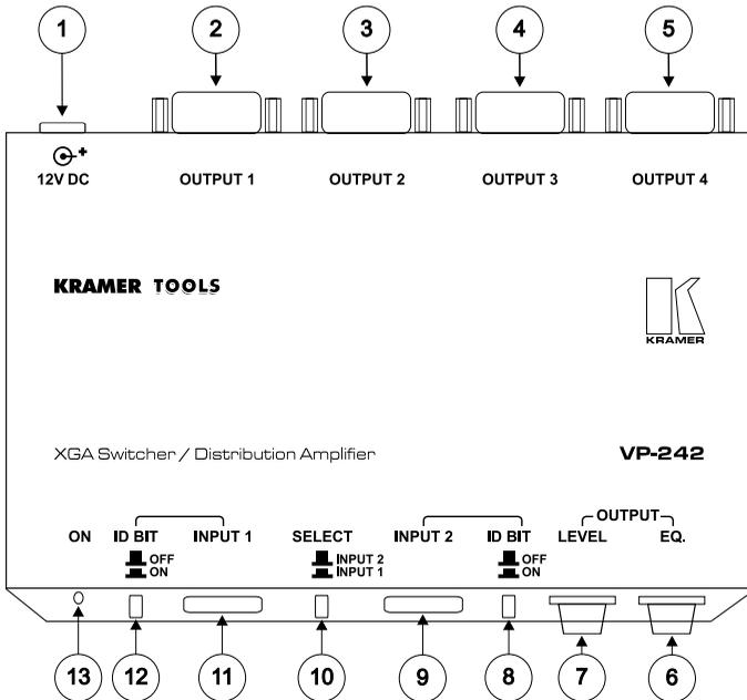
Figure 1: VP-242 XGA Switcher / Distribution Amplifier
