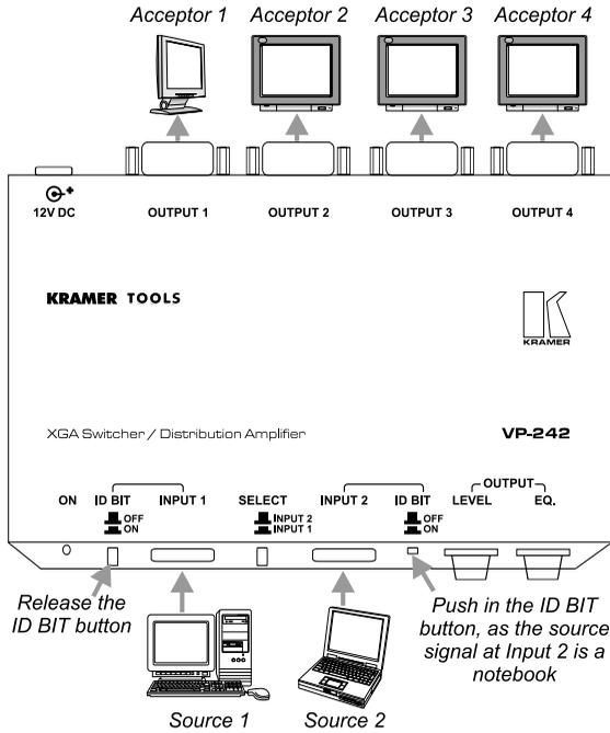
*Figure 2: VP-242 XGA Switcher / Distribution Amplifier Connections*
