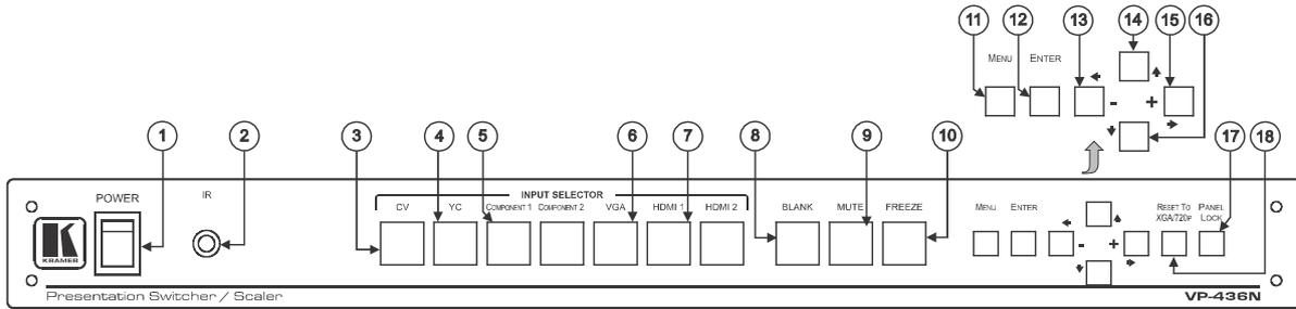
Figure 1: VP-436N Presentation Switcher/Scaler Front Panel
