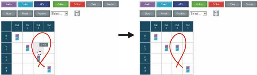
Figure 17: Switching an Input to an Output
