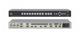
The VP-731 is a 9-input scaler/switcher for analog video, digital video, balanced stereo and S/PDIF audio signals. It up or down-scales composite, s-Video (Y/C), component video (YUV), HDMI, computer graphics video and JPEG files to a selectable computer graphics video or HDTV output resolution on one HDMI and two 15-pin HD outputs. The VP-731 is the same as the VP-730 with the addition of Ethernet control.
