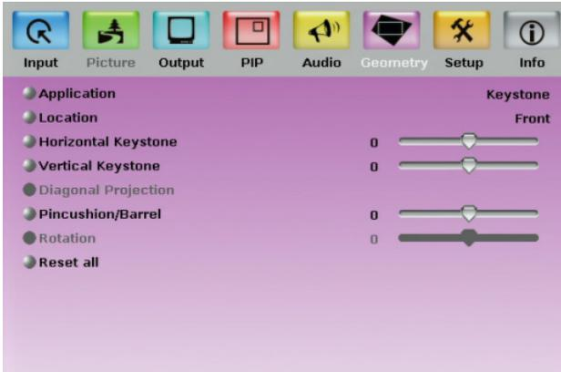
Figure 19: Geometry Screen
