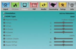
The **VP-731** is set at the factory to a default output resolution of 1024x768 (XGA) with a refresh rate of 60Hz.
