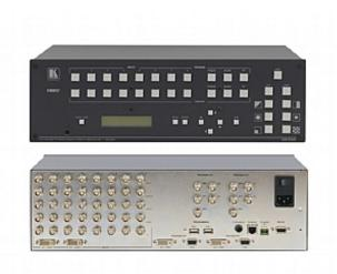
The VP-747 In-CTRL Dual Scaler Seamless Switcher is a true multi-standard scaler and seamless switcher with 8 universal inputs comprised of 5 BNCs each, any of which accommodate can а composite video, s-Video (Y/C), component video (RGB/YUV), RGBS, or RGBHV signal. Inputs 1 and 2 also can be configured to HDMI/DVI inputs. The unit has dual scalers, one for the preview and the other for the program output. Dual scalers are required to do "true" seamless transitions from one source to another.
