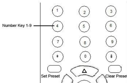
1、Preset setting : to set a preset position, the users should press the "【SET PRESET】" key first and then press the number key 0-9 to set a relative preset, 10 preset positions in total are available.
