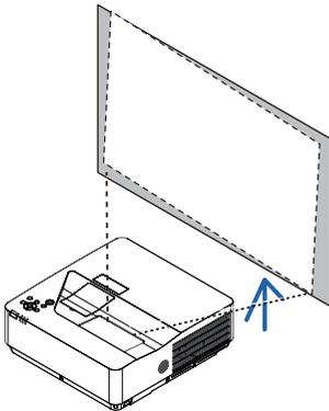
Adjusting the throw angle (the height of an image) [Tilt foot]
