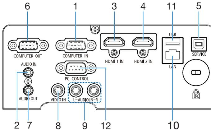
1. **COMPUTER IN/ Component Input Terminal (Mini D-Sub 15 Pin)**
