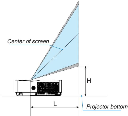
(Note) Height from lens center to lower edge of screen (with tilt feet screwed in)
