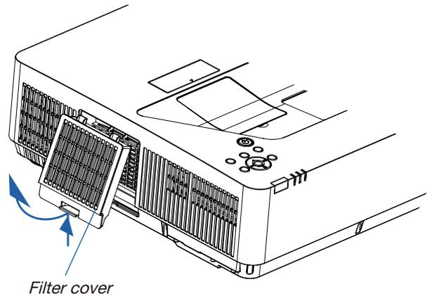
2. Vacuum dust on the front and back faces of the filter unit.
