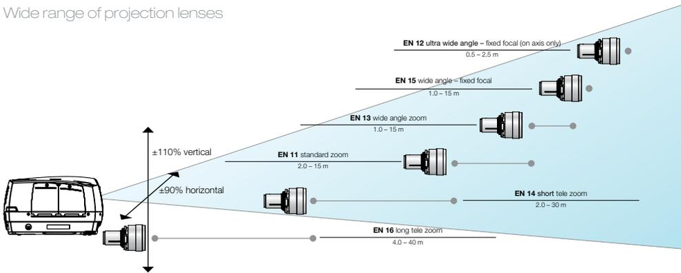
Multiple lens options and very wide lens shift adjustment ranges allow for flexibility in installations.
