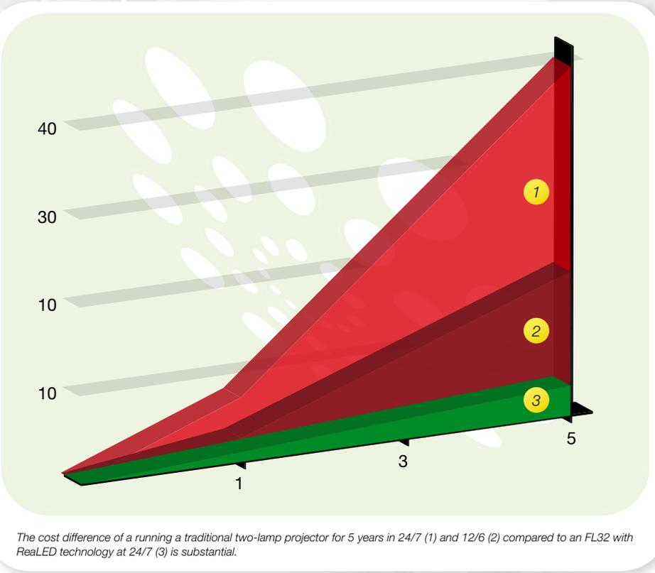
The cost difference of a running a traditional two-lamp projector for 5 years in 24/7 (1) and 12/6 (2) compared to an FL32 with ReaLED technology at 24/7 (3) is substantial.
