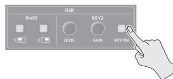
The KEY1 [KEY ON] or KEY2 [KEY ON] button lights up in green, and a preview of the composition results is displayed in the PVW section of the multi-view monitor.
