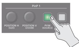
The PinP 1 [PVW] button lights up in green and the inset screen appears in the PVW section of the monitor, allowing you to check the inset screen's location and size.
