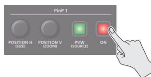
The PinP 1 [ON] button lights up in red, and the inset screen is composited onto the background video and the result is sent to final output.
