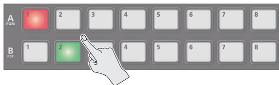
2. Press the SPLIT/VFX [A] or [B] button to turn on the visual effect (making the button light up).
