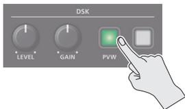
The DSK [PVW] button lights up in green, and a preview of the composition results is displayed in the PVW section of the monitor.
