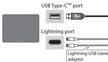
You can use a commercially available connection cable or adaptor cable (Lightning-USB camera adaptor) to connect an iPad, and remotely control the V-8HD.
