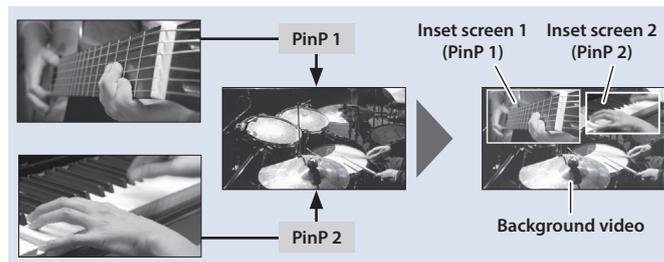
Here we explain the procedure for compositing video using "PinP 1." You can also composite video using the same procedure using "PinP 2."
