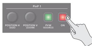
The PinP 1 [ON] button lights up in red, and the inset screen is composited onto the background video and the result is sent to final output.
