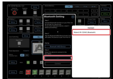
\* Although you may configure the device to pair with multiple VR-120HD units, the device can only pair with one VR-120HD at a time.
