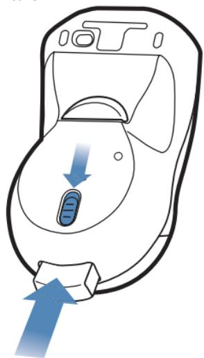
**15** Insert the USB Receiver into the USB storage compartment. Push gently until it clicks in place. Push gently again to release.
